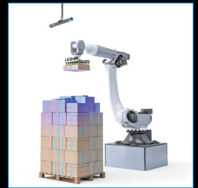
Depalletization of unstructured box shipments - handling mixed sizes, shapes, and orientations with robotic precision.
