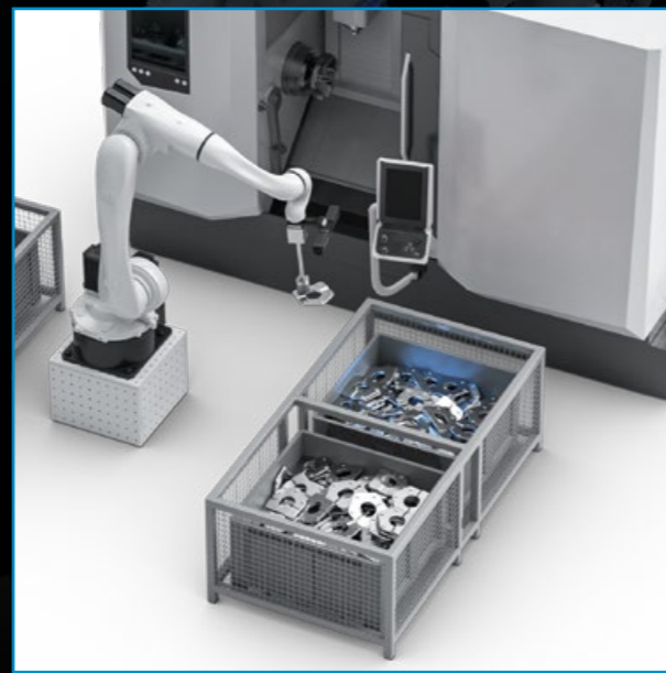
Machine tending - load, unload, and inspect parts in CNC or injection molding cells - handling raw, unfinished, or variable workpieces.
