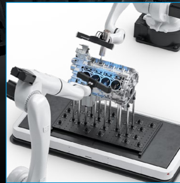
Part inspection - submillimeter accuracy for inspecting complex geometries - detecting defects, verifying tolerances, and ensuring quality control.
