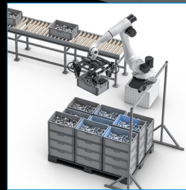
Tote identification and depalletization automating high-volume logistics with unmatched speed and accuracy.
